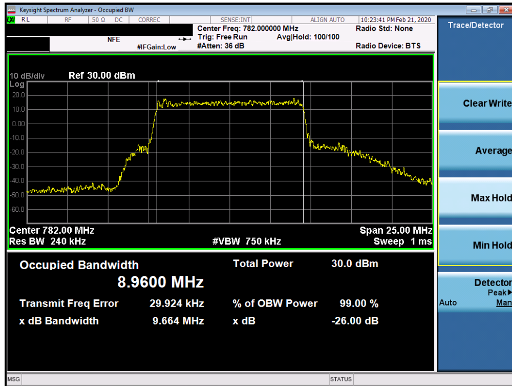
Plot 7-17. Occupied Bandwidth Plot (Band 13 - 10.0MHz 16-QAM - Full RB Configuration)
