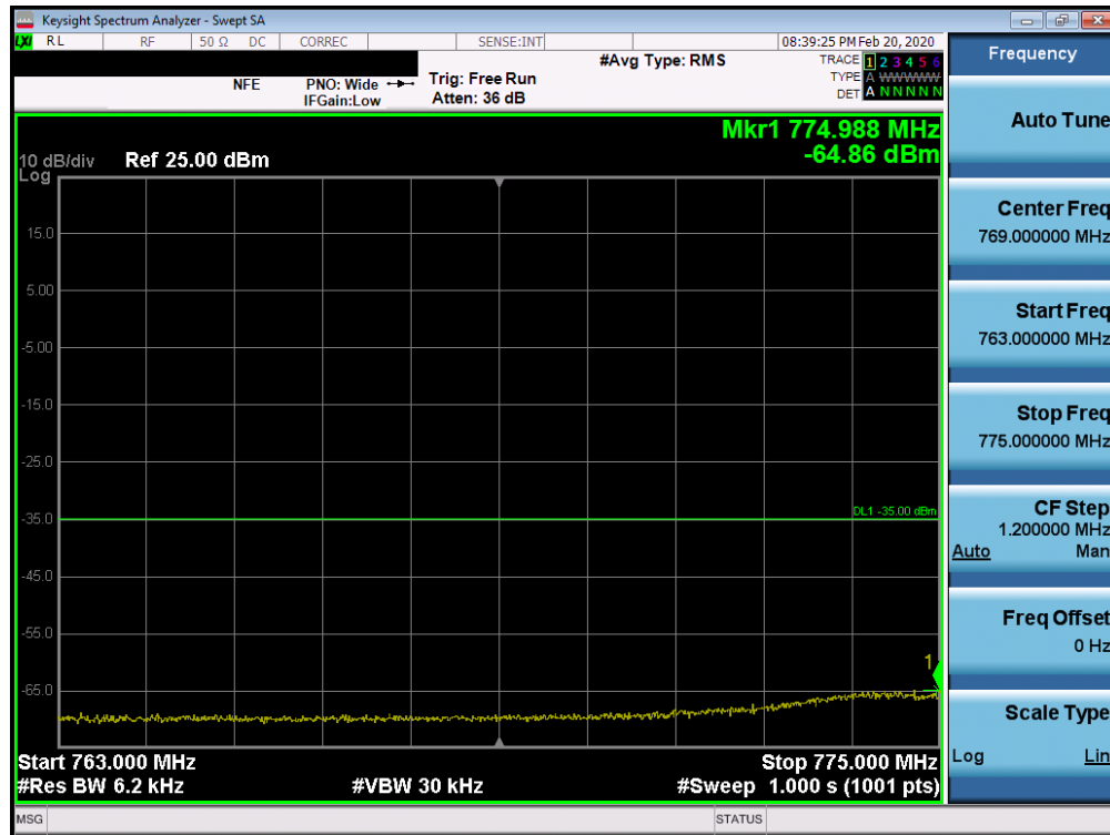
Plot 7-142. Lower Emission Mask Plot (Band 13 - 10.0MHz QPSK - Full RB Configuration)
