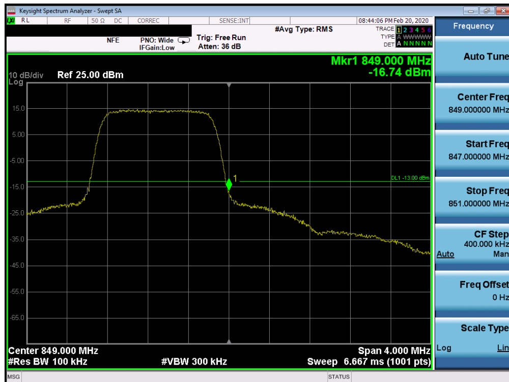
Plot 7-146. Upper Band Edge Plot (Band 5 - 1.4MHz QPSK - Full RB Configuration)
