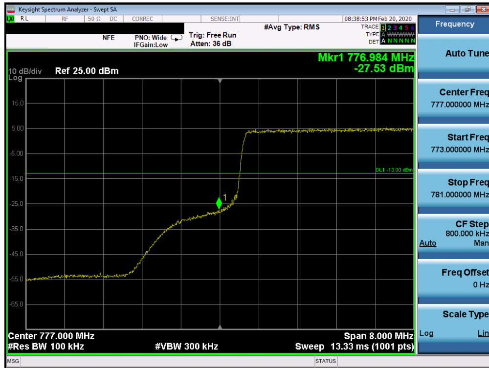
Plot 7-141. Lower Band Edge Plot (Band 13 - 10.0MHz QPSK - Full RB Configuration)
