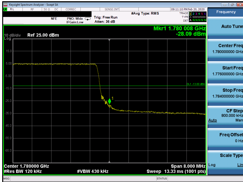
Plot 7-175. Upper Band Edge Plot (Band 66 - 10.0MHz QPSK - Full RB Configuration)
