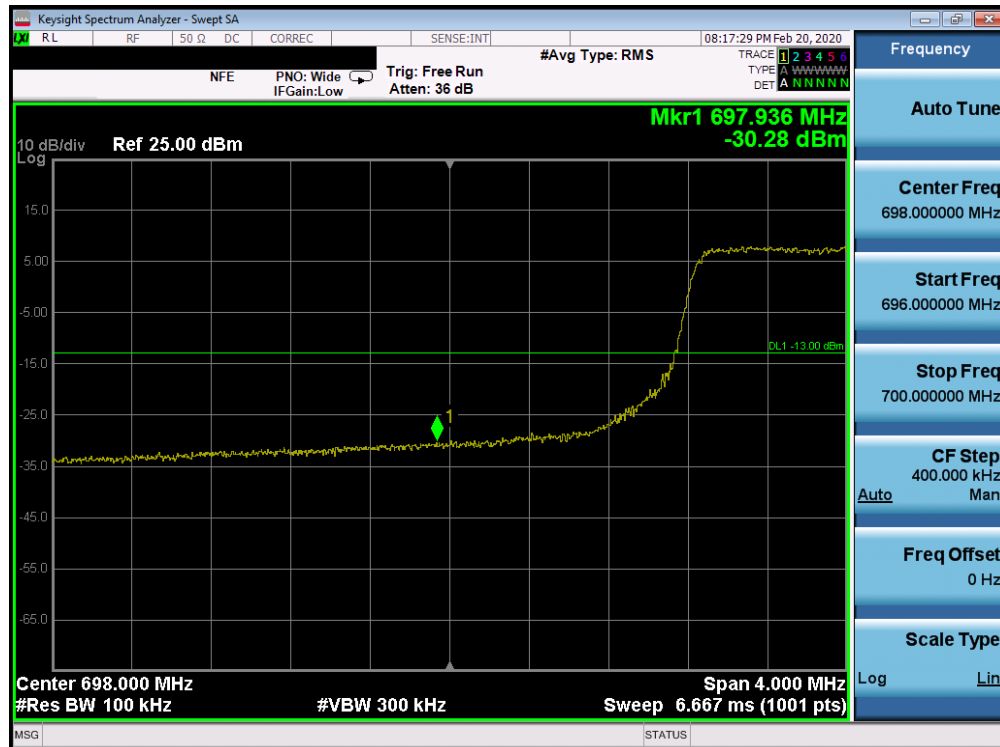
Plot 7-131. Lower Band Edge Plot (Band 12 - 5.0MHz QPSK - Full RB Configuration)
