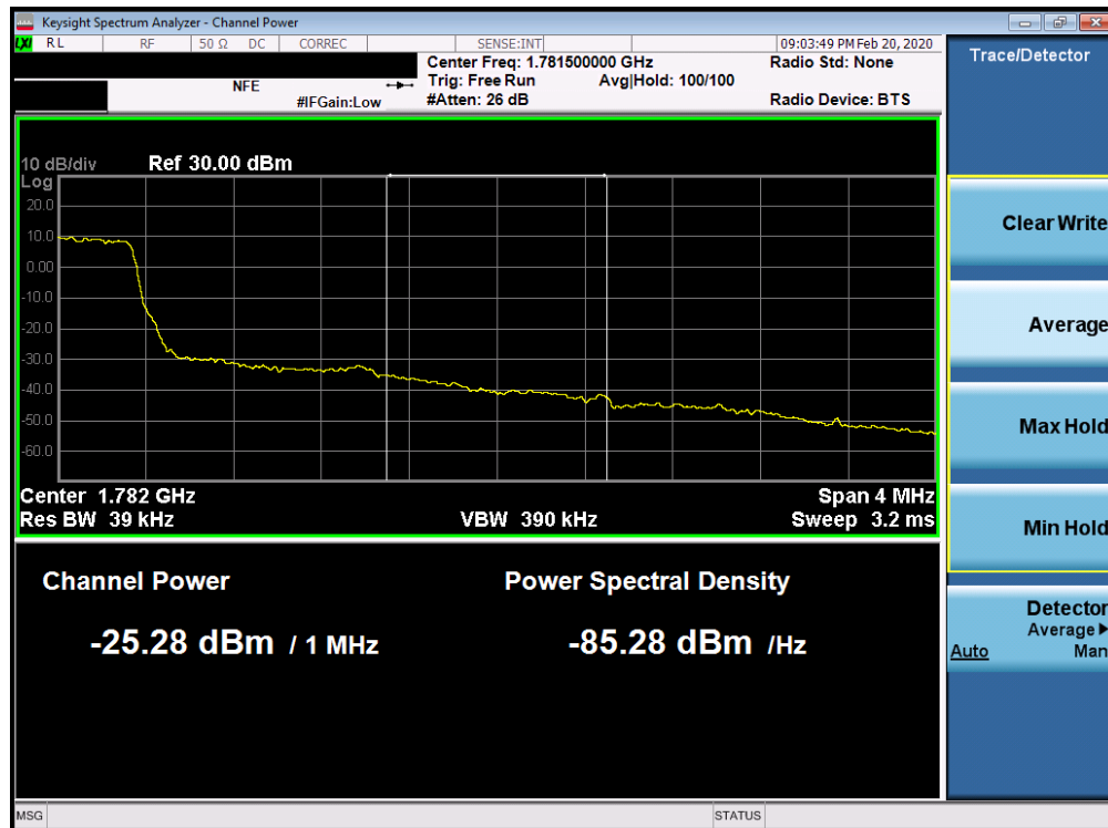
Plot 7-158. Upper Extended Band Edge Plot (Band 66 - 1.4MHz QPSK - Full RB Configuration)
