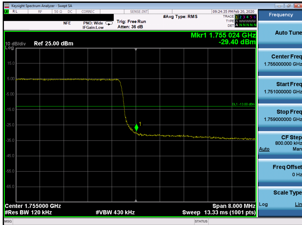
Plot 7-173. Upper Band Edge Plot (Band 4 - 10.0MHz QPSK - Full RB Configuration)
