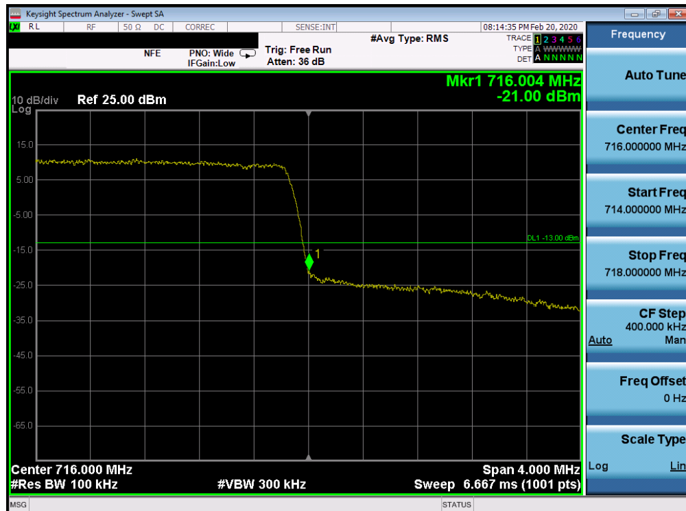
Plot 7-130. Upper Band Edge Plot (Band 12 - 3.0MHz QPSK - Full RB Configuration)
