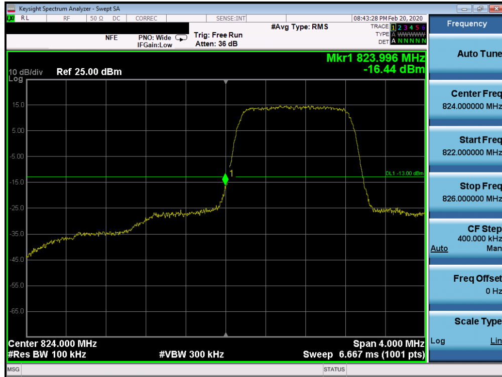
Plot 7-145. Lower Band Edge Plot (Band 5 - 1.4MHz QPSK - Full RB Configuration)
