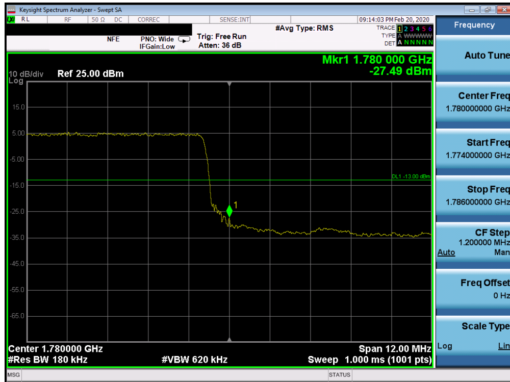
Plot 7-181. Upper Band Edge Plot (Band 66 - 15.0MHz QPSK - Full RB Configuration)
