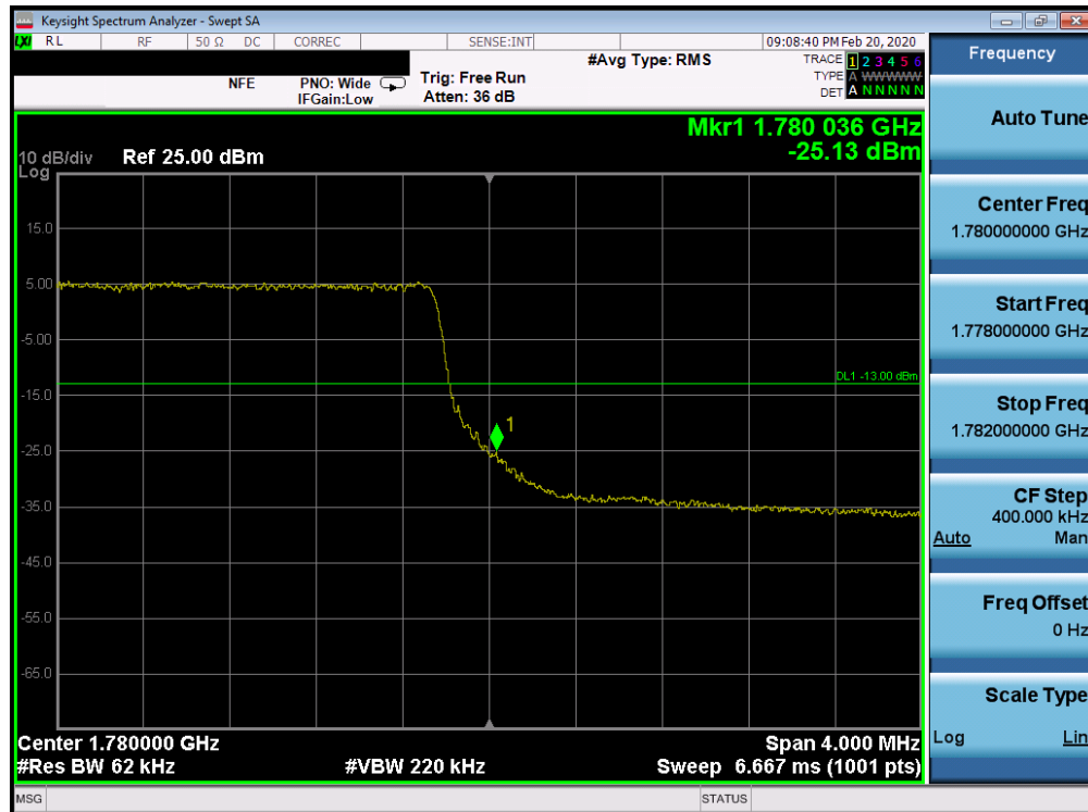
Plot 7-169. Upper Band Edge Plot (Band 66 - 5.0MHz QPSK - Full RB Configuration)
