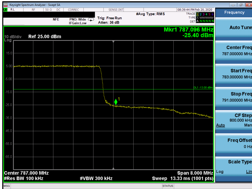
Plot 7-143. Upper Band Edge Plot (Band 13 - 10.0MHz QPSK - Full RB Configuration)
