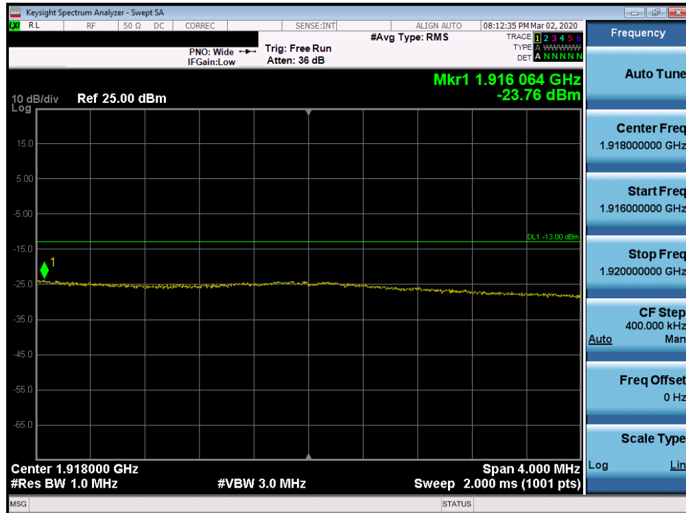
Plot 7-218. Upper Extended Band Edge Plot (Band 25 - 15.0MHz QPSK - Full RB Configuration)
