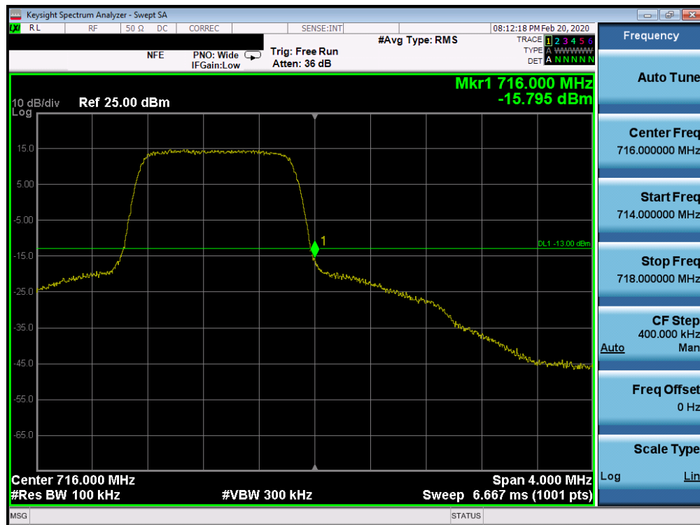
Plot 7-128. Upper Band Edge Plot (Band 12 - 1.4MHz QPSK - Full RB Configuration)
