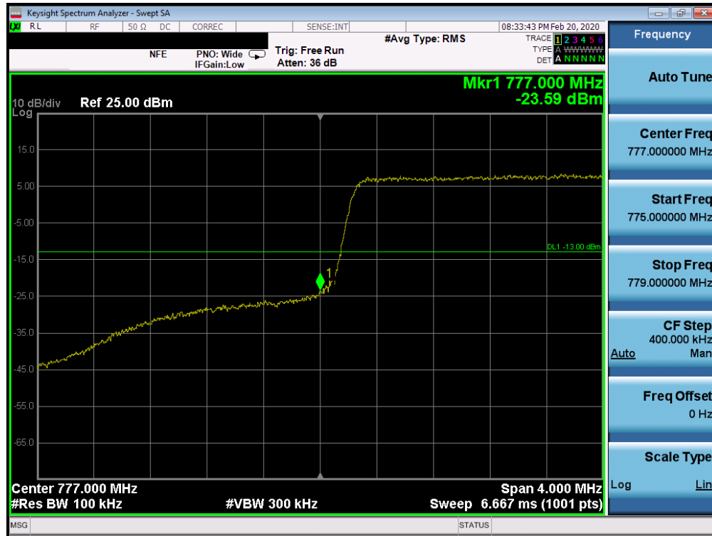
Plot 7-137. Lower Band Edge Plot (Band 13 - 5.0MHz QPSK - Full RB Configuration)
