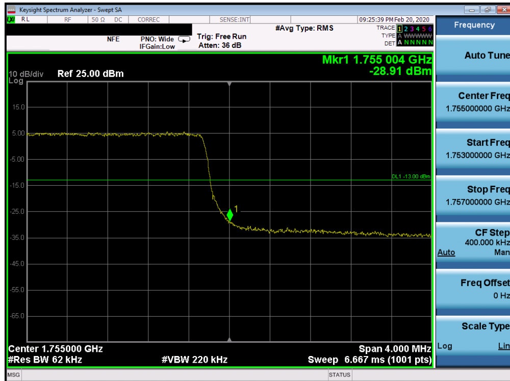
Plot 7-167. Upper Band Edge Plot (Band 4 - 5.0MHz QPSK - Full RB Configuration)
