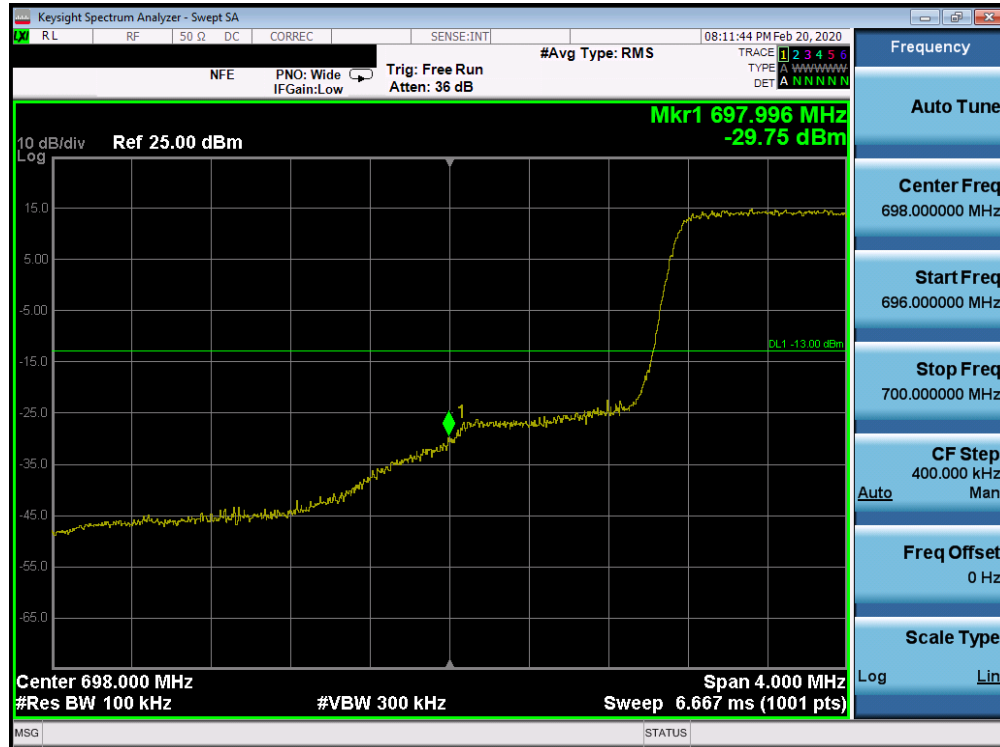
Plot 7-127. Lower Band Edge Plot (Band 12 - 1.4MHz QPSK - Full RB Configuration)
