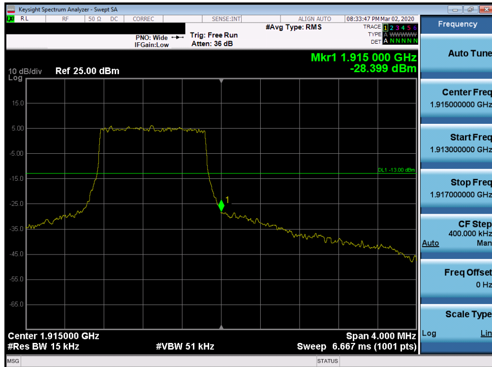
Plot 7-193. Upper Band Edge Plot (Band 25 - 1.4MHz QPSK - Full RB Configuration)
