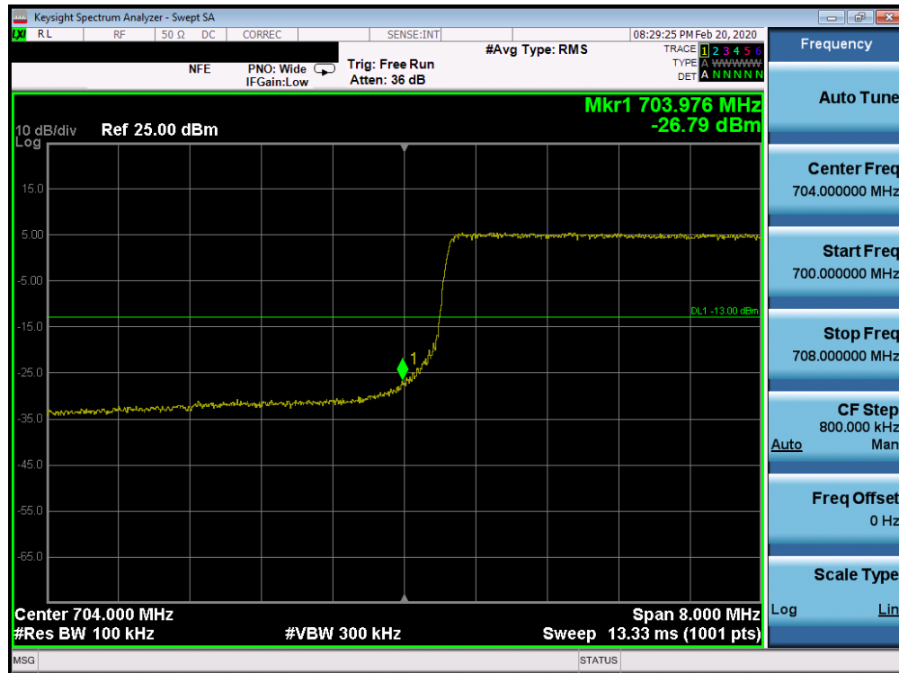
Plot 7-135. Lower Band Edge Plot (Band 17 - 10.0MHz QPSK - Full RB Configuration)
