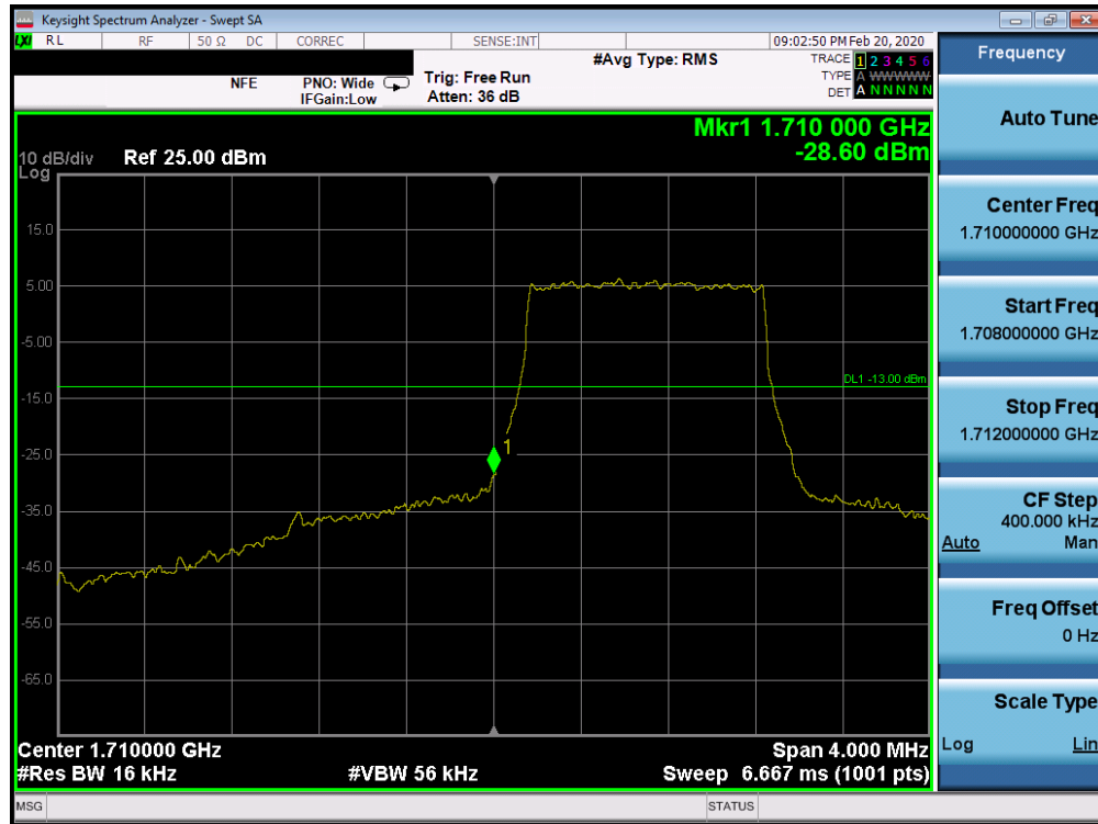
Plot 7-153. Lower Band Edge Plot (Band 66/4 - 1.4MHz QPSK - Full RB Configuration)
