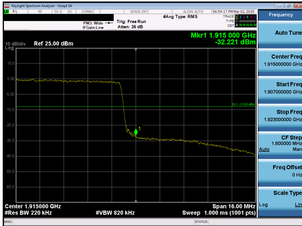
Plot 7-223. Upper Band Edge Plot (Band 25 - 20.0MHz QPSK - Full RB Configuration)
