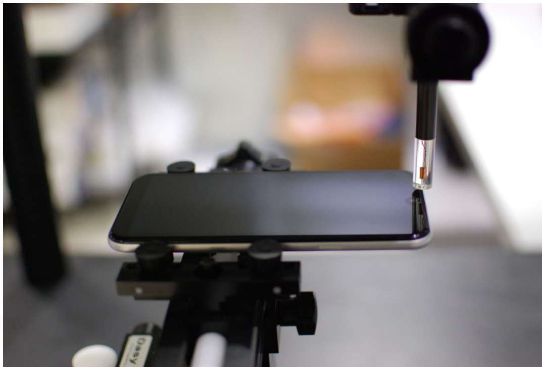
Figure 15-1 Test Setup for Wireless Device
