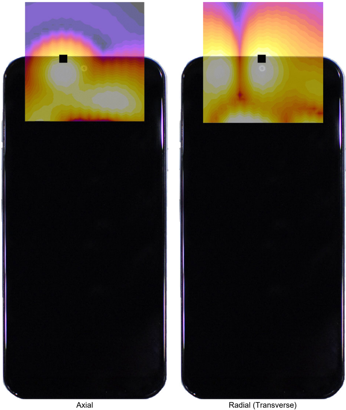
Figure 15-3 T-Coil Scan Overlay Magnetic Field Distributions
