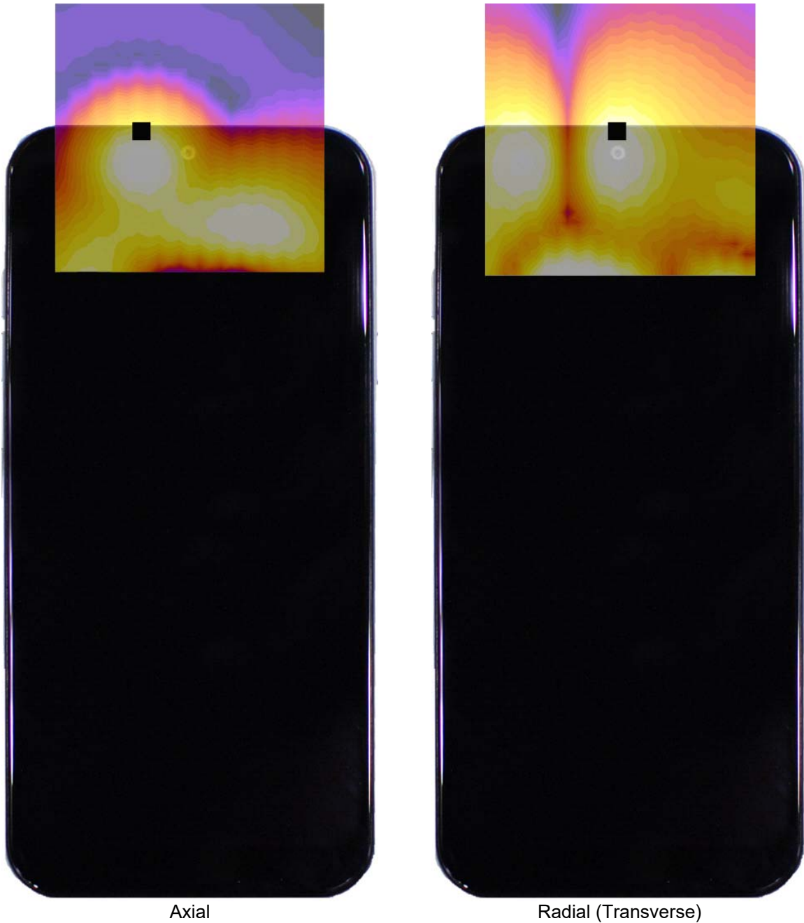
Figure 13-3 T-Coil Scan Overlay Magnetic Field Distributions
