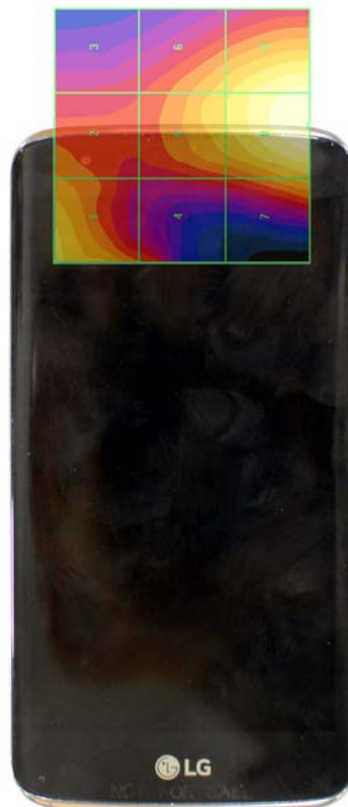
Figure 18-4 E-Field WD Scan overlay
