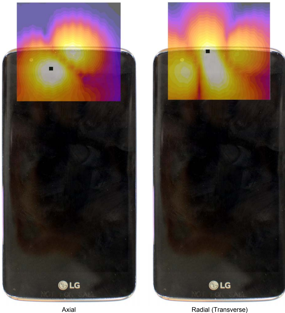
Figure 13-3 T-Coil Scan Overlay Magnetic Field Distributions
