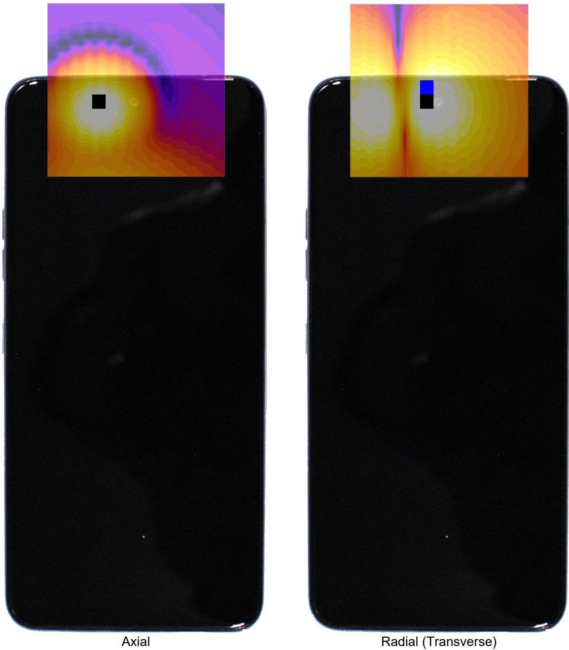
Figure 16-3 T-Coil Scan Overlay Magnetic Field Distributions
