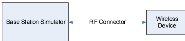
Figure 9-1 Power Measurement Setup
