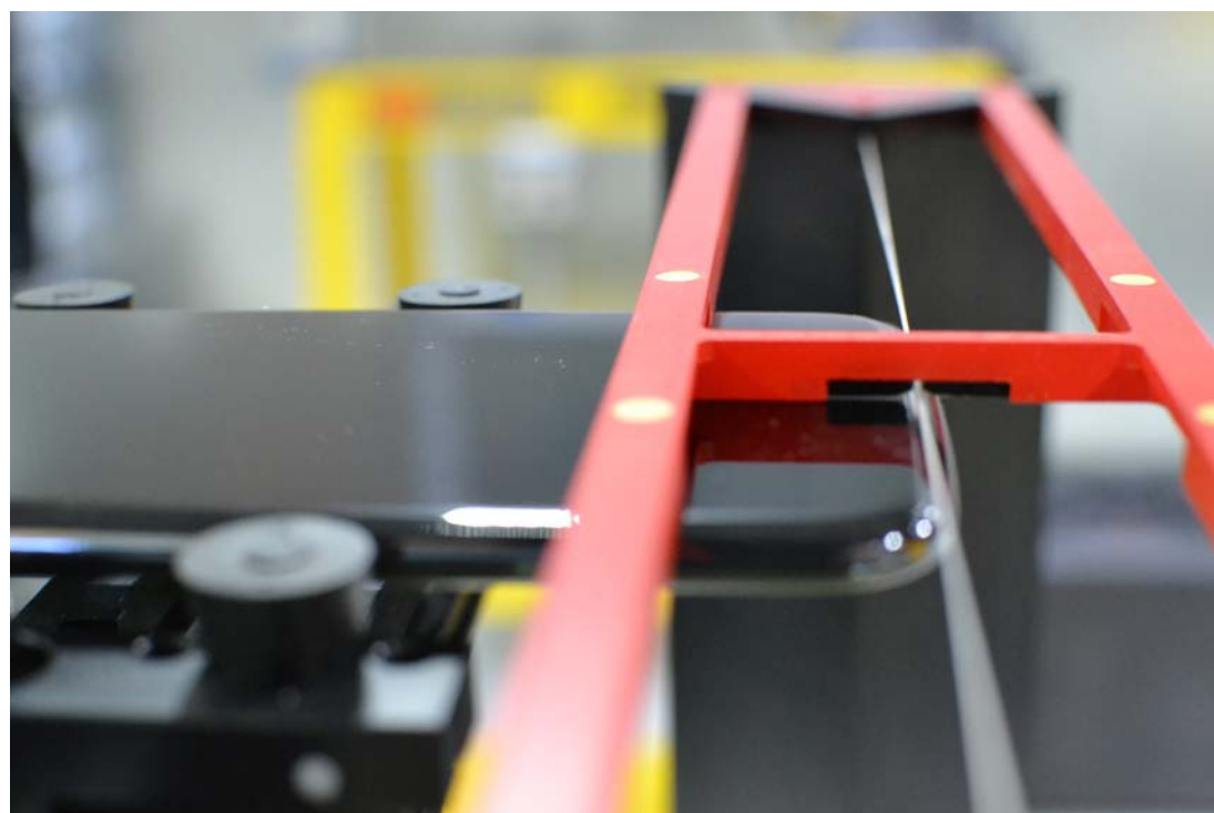
Figure 18-2 HAC Phantom Plane Alignment
