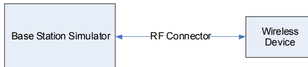
Figure 9-1 Power Measurement Setup
