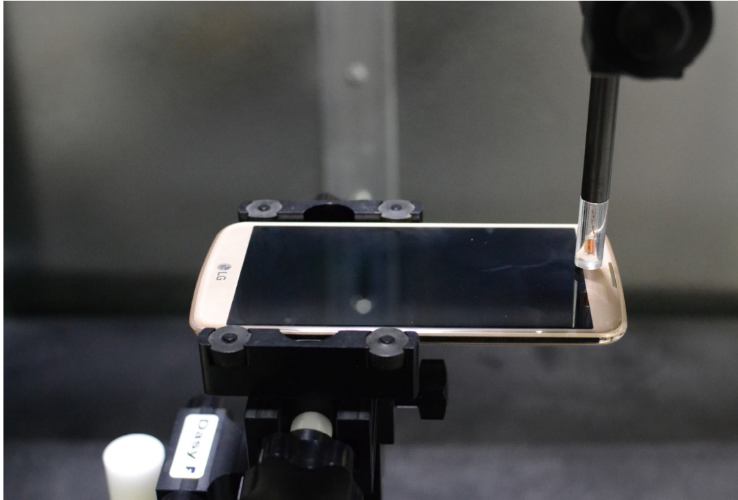
Figure 14-1 Test Setup for Wireless Device
