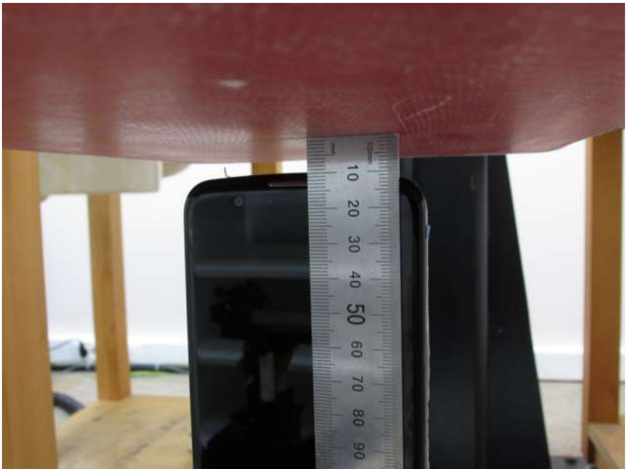
[Distance of 1.0 cm from the EUT]
