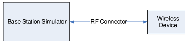
Figure 9-3 Power Measurement Setup
