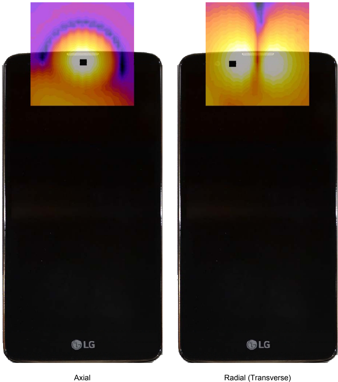
Figure 14-3 T-Coil Scan Overlay Magnetic Field Distributions
