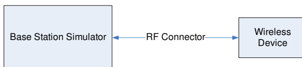
Figure 9-3 Power Measurement Setup
