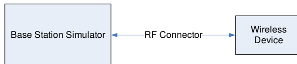
Figure 9-2 Power Measurement Setup
