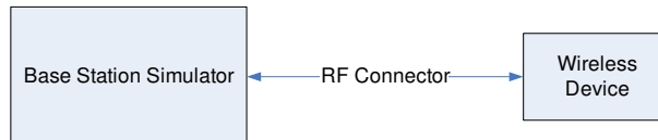
Figure 9-1 Power Measurement Setup
