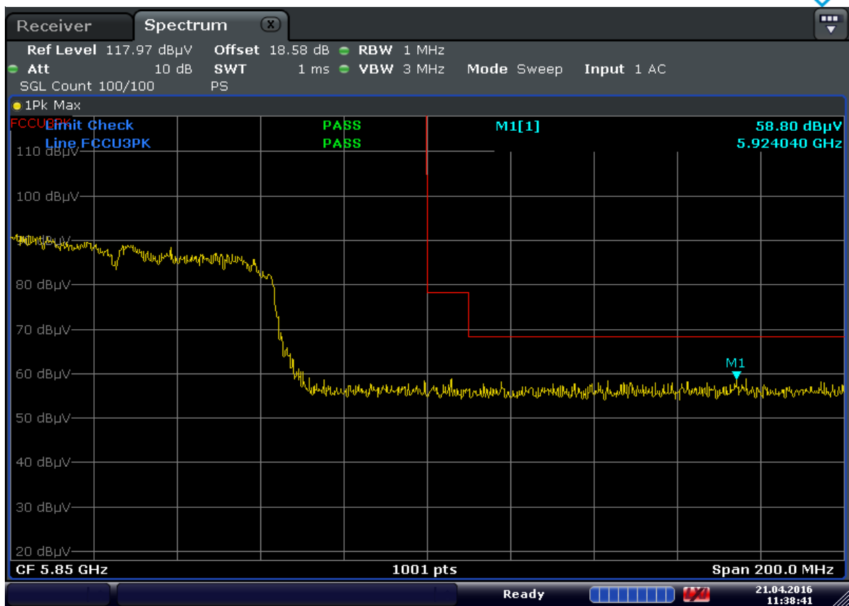
Plot 7-112. Radiated Upper Band Edge Plot (Peak – UNII Band 3)
