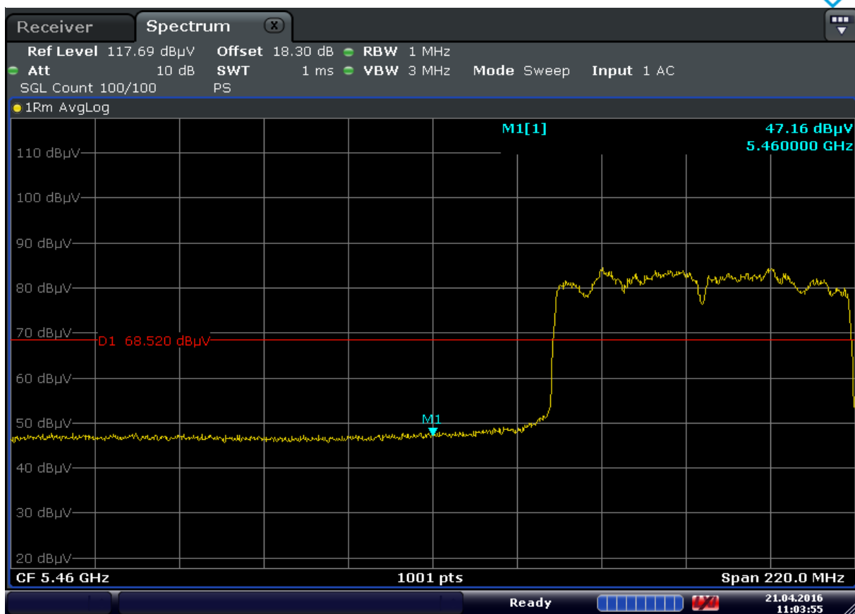
Plot 7-109. Radiated Restricted Lower Band Edge Plot (Average – UNII Band 2C)
