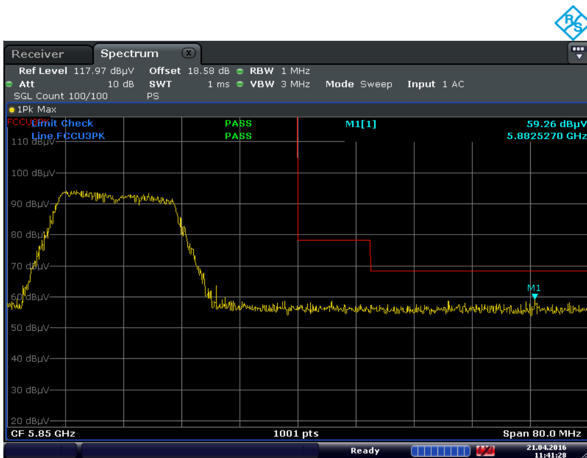
Plot 7-95. Radiated Upper Band Edge Plot (Peak – UNII Band 3)
