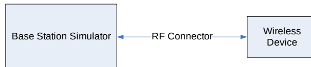
Figure 9-2 Power Measurement Setup
