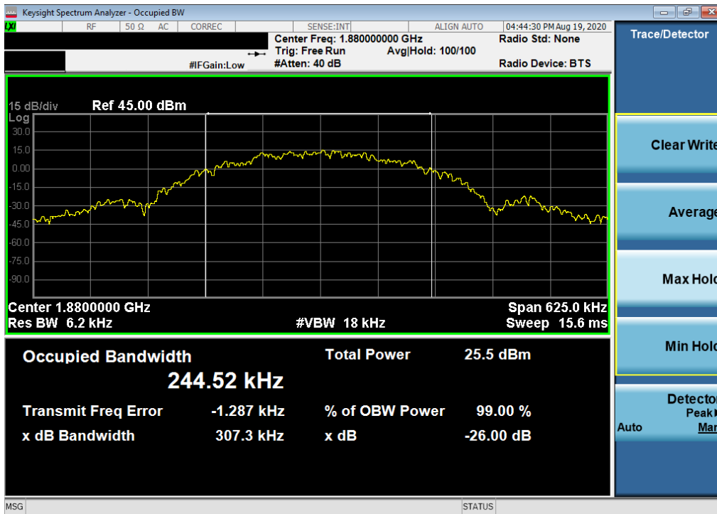
Plot 7-4. Occupied Bandwidth Plot (PCS EDGE Mode)
