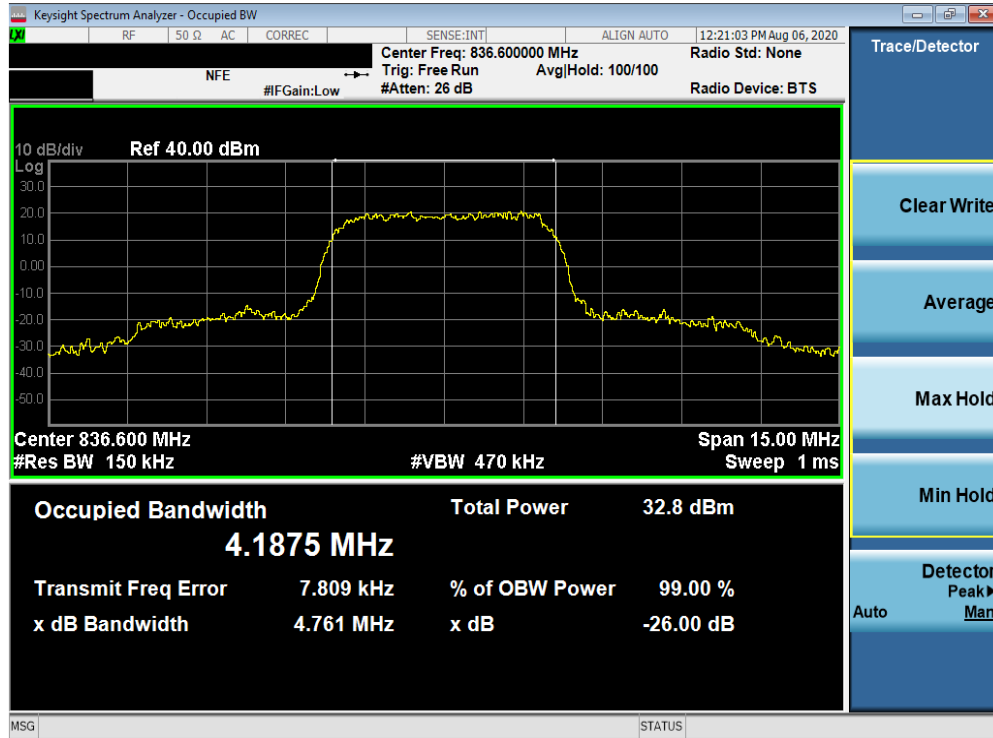
Plot 7-7. Occupied Bandwidth Plot (Cellular WCDMA Mode)
