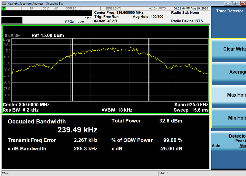
Plot 7-3. Occupied Bandwidth Plot (Cellular EDGE Mode)
