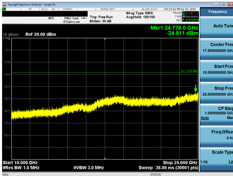
Plot 7-39. Conducted Spurious Plot (Bluetooth, 3Mbps – Ch. 39)
