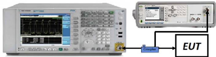
Figure 7-2. Test Instrument & Measurement Setup
