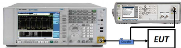
Figure 7-1. Test Instrument & Measurement Setup
