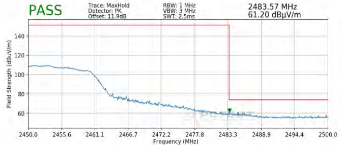
Plot 7-102. Radiated Restricted Upper Band Edge Measurement SISO ANT1 (Peak)
