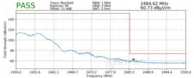
Plot 7-110. Radiated Restricted Upper Band Edge Measurement SISO ANT1 (Peak)
