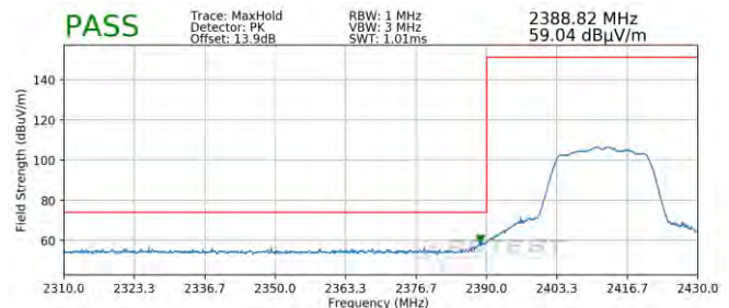
Plot 7-98. Radiated Restricted Lower Band Edge Measurement SISO ANT2 (Peak)
