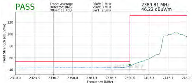
Plot 7-99. Radiated Restricted Lower Band Edge Measurement SISO ANT1 (Average)
