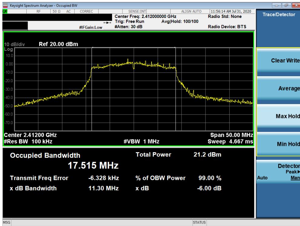
Plot 7-19. 6dB Bandwidth Plot SISO ANT2 (802.11n (2.4GHz) – Ch. 1)
