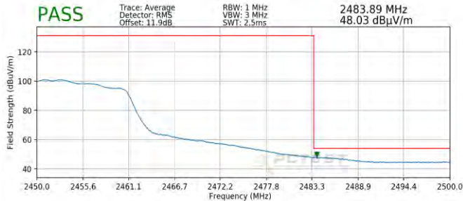
Plot 7-101. Radiated Restricted Upper Band Edge Measurement SISO ANT1 (Average)
