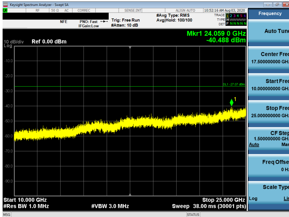
Plot 7-76. Conducted Spurious Plot SISO ANT2 (802.11b – Ch. 11)
