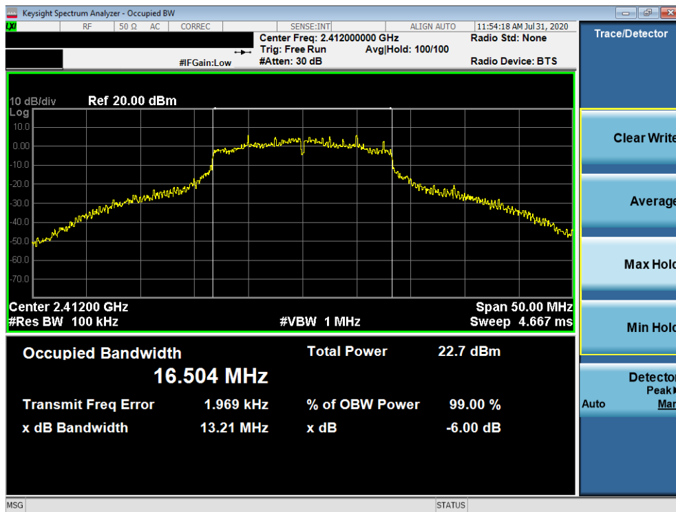
Plot 7-16. 6dB Bandwidth Plot SISO ANT2 (802.11g – Ch. 1)
