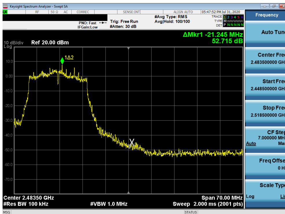
Plot 7-56. Band Edge Plot SISO ANT1 (802.11ac (2.4GHz) – Ch. 11)
