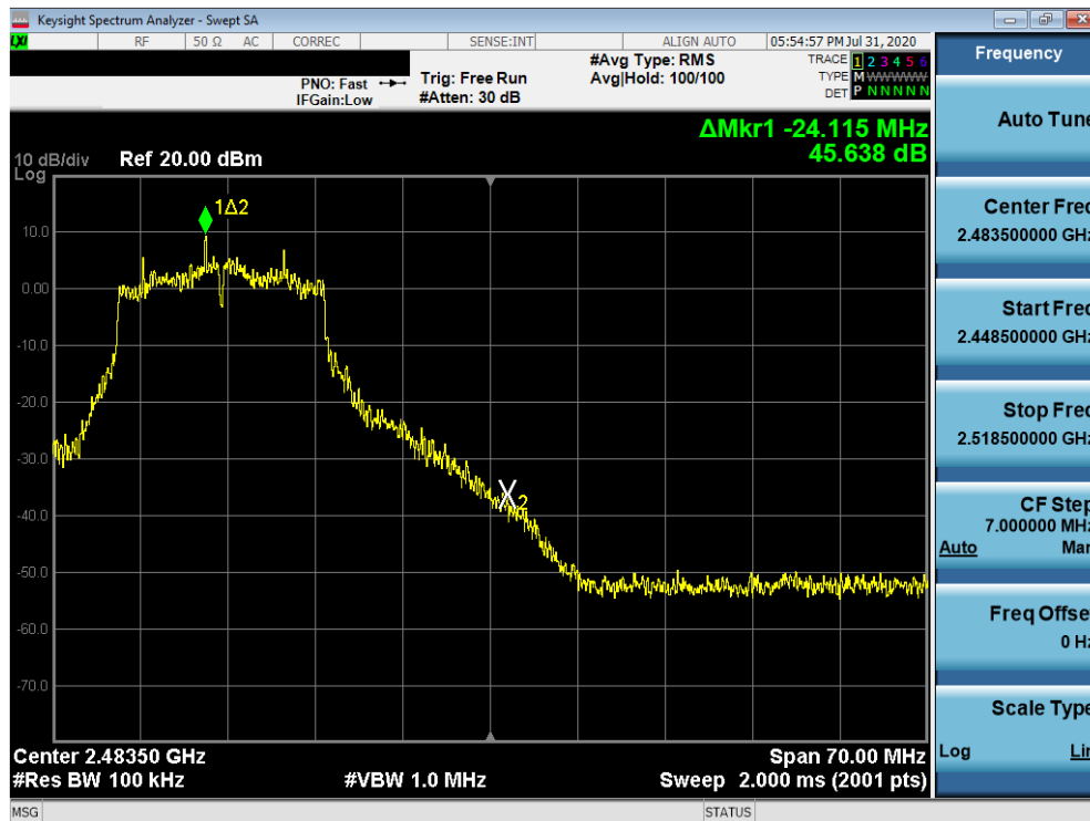
Plot 7-60. Band Edge Plot SISO ANT2 (802.11g – Ch. 11)
