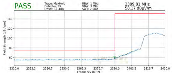
Plot 7-100. Radiated Restricted Lower Band Edge Measurement SISO ANT1 (Peak)
