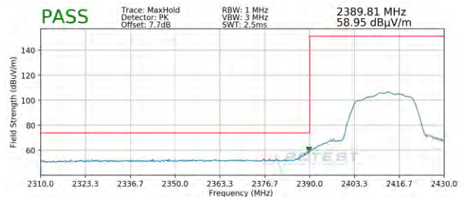
Plot 7-90. Radiated Restricted Lower Band Edge Measurement SISO ANT1 (Peak)
