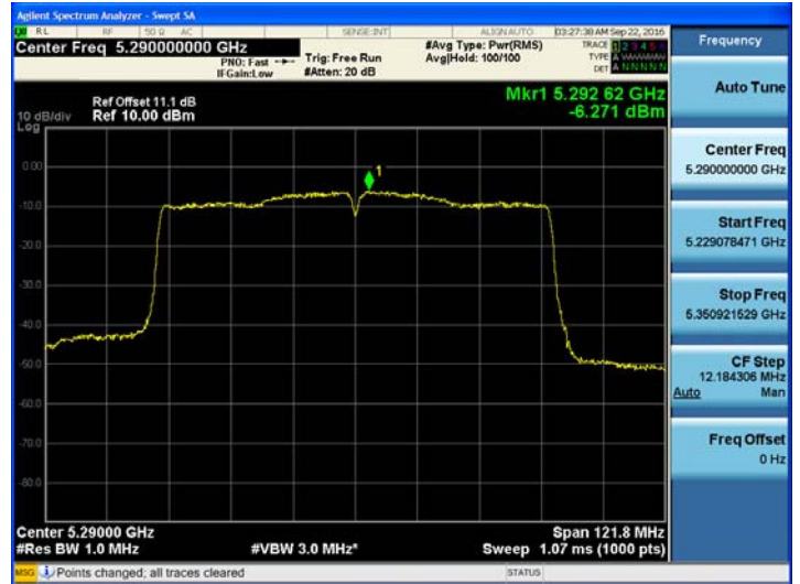
802.11ac_VHT80 UNII 3 BAND PSD CH 155
