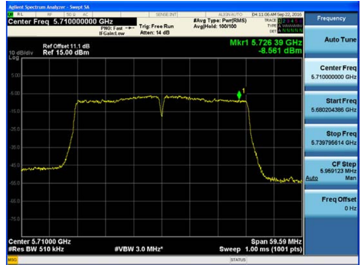
802.11ac_VHT40 UNII 3 Band PSD CH.142
