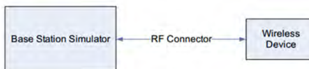
Figure 9.1 Power Measurement Setup
