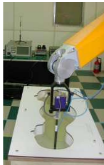
Figure 4.1 Photograph of the probe and the Phantom
