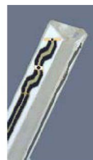
Figure 3.3 Probe Thick-Film Technique
