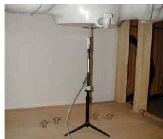
Figure 11.1 Dipole Verification Test Setup Diagram & Photo
