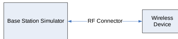
Figure 8-2 Power Measurement Setup
