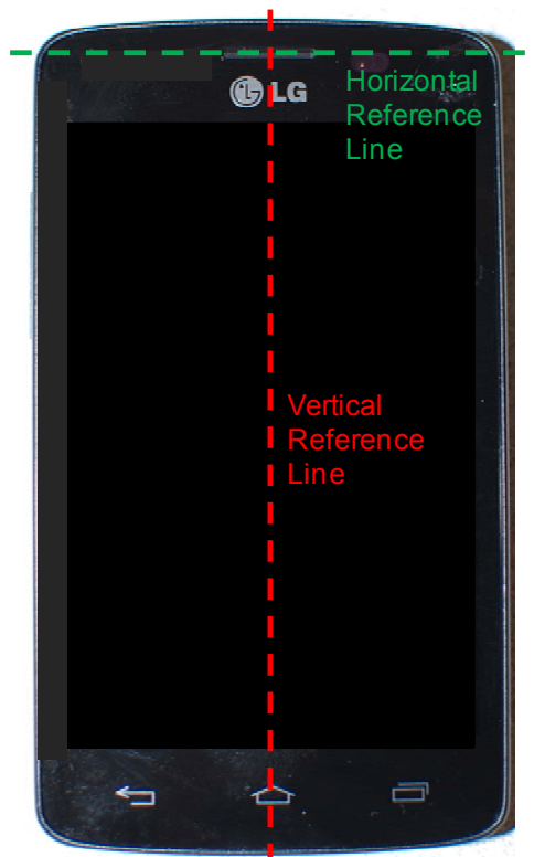
SAR Test Setup Photo 6 – Vertical and Horizontal Reference Lines
