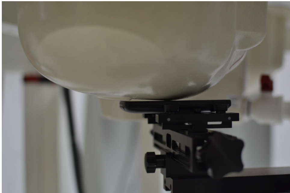
SAR Test Setup Photo 1 – Right Cheek
