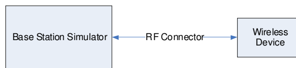
Figure 8-1 Power Measurement Setup
