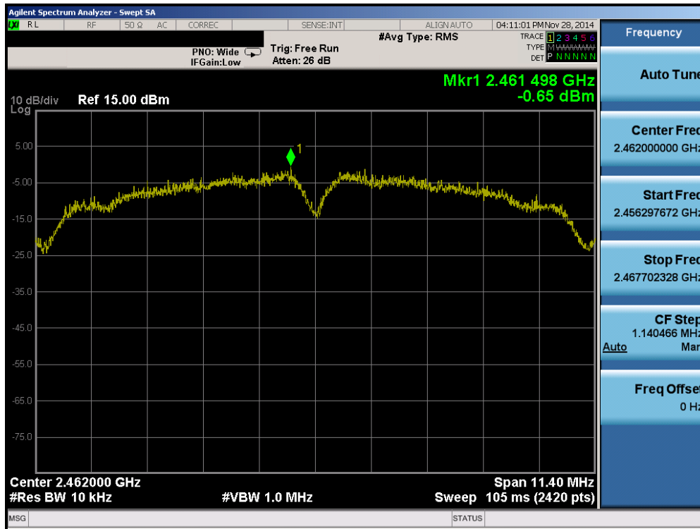
Plot 6-12. Power Spectral Density Plot (802.11b – Ch. 11)
