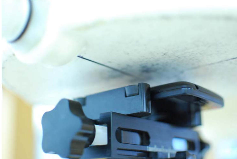
SAR Test Setup Photo 5 – Body-worn at 15mm
