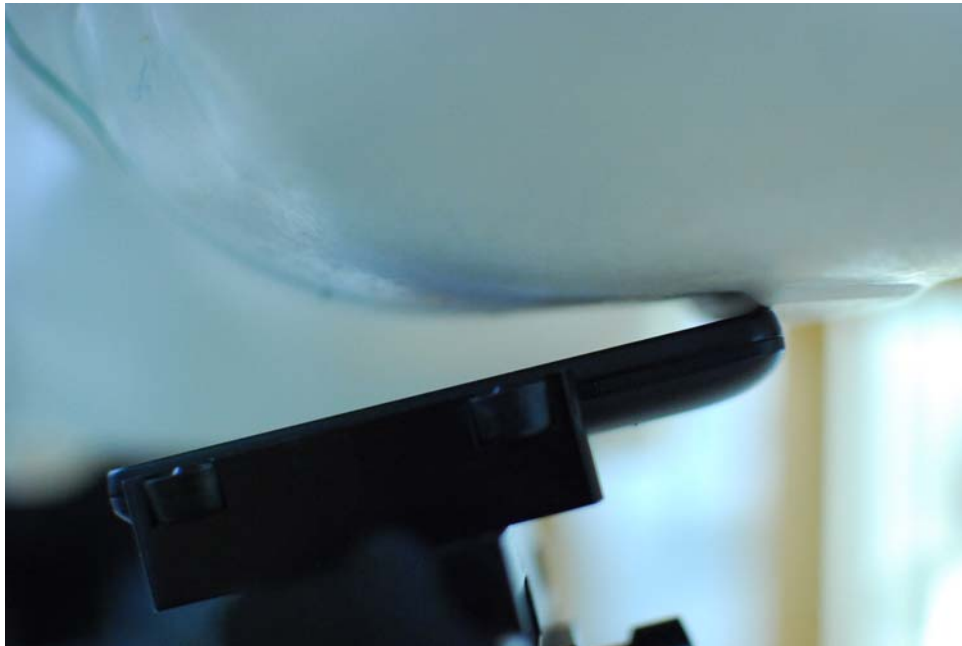
SAR Test Setup Photo 4 – Left Tilt
