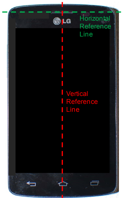
SAR Test Setup Photo 6 – Horizontal and Vertical Reference Lines
