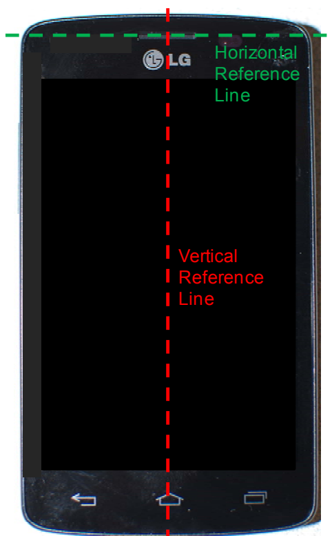
SAR Test Setup Photo 6 – Horizontal and Vertical Reference Lines
