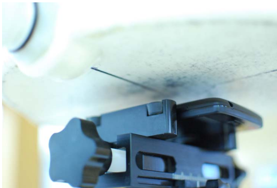
SAR Test Setup Photo 5 – Body-worn at 15mm
