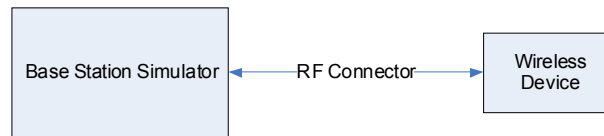
Figure 8-1 Power Measurement Setup
