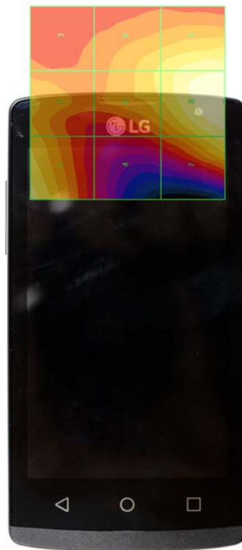
Figure 18-4 E-Field WD Scan overlay
