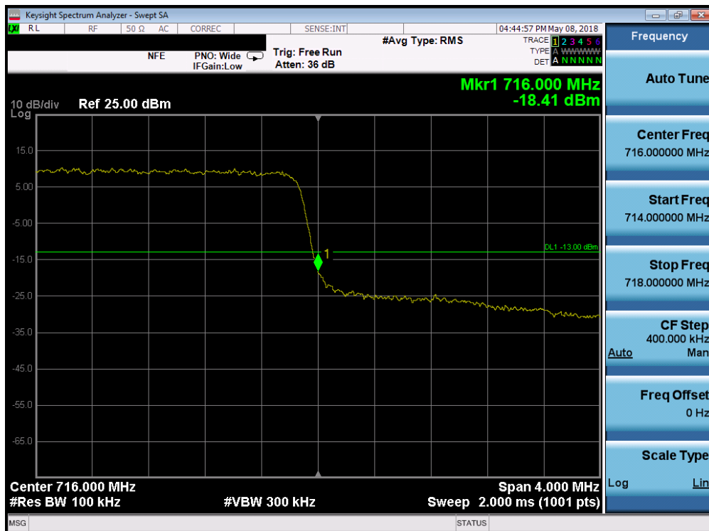
Plot 7-105. Upper Band Edge Plot (Band 12 - 3.0MHz QPSK - Full RB Configuration)
