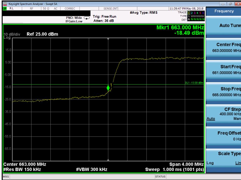
Plot 7-94. Lower Band Edge Plot (Band 71 - 5.0MHz QPSK - Full RB Configuration)
