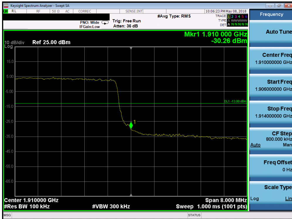
Plot 7-168. Upper Band Edge Plot (Band 2 - 10.0MHz QPSK - Full RB Configuration)
