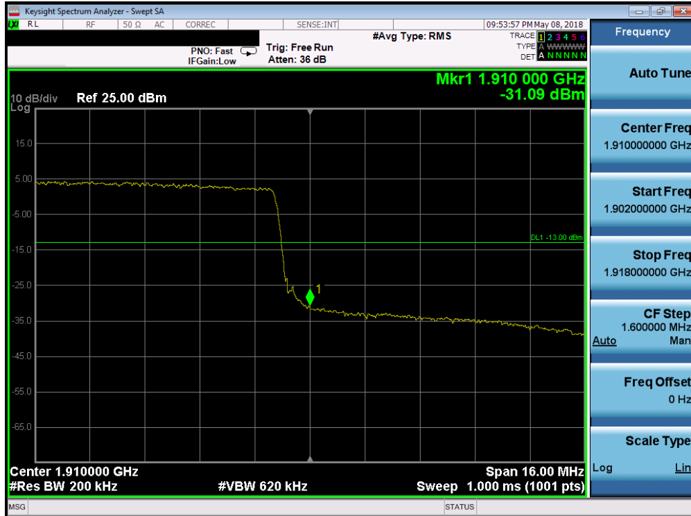
Plot 7-176. Upper Band Edge Plot (Band 2 - 20.0MHz QPSK - Full RB Configuration)
