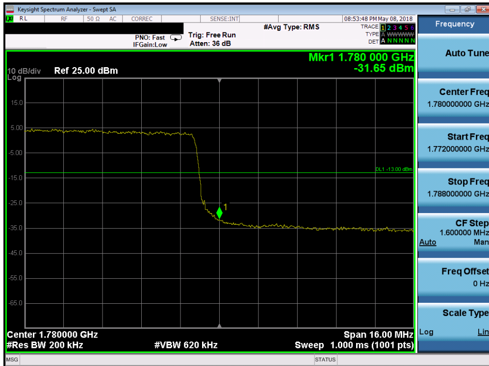
Plot 7-152. Upper Band Edge Plot (Band 66 - 20.0MHz QPSK - Full RB Configuration)
