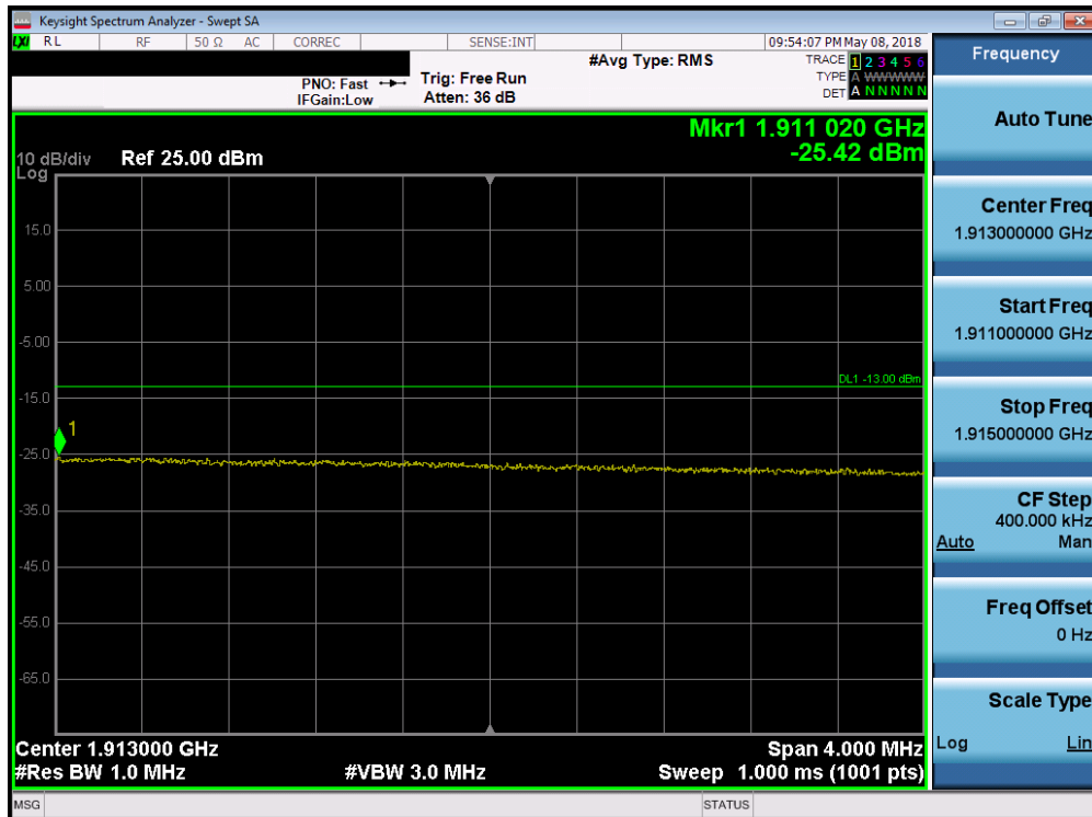
Plot 7-177. Upper Extended Band Edge Plot (Band 2 - 20.0MHz QPSK - Full RB Configuration)
