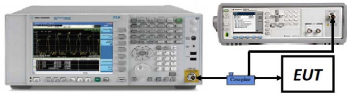
Figure 7-4. Test Instrument & Measurement Setup
