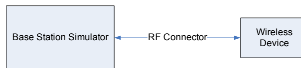
Figure 8-2 Power Measurement Setup
