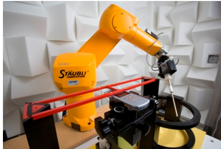
Figure 4-3 SPEAG Robotic System
