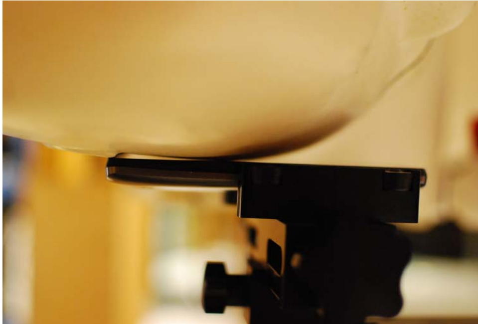
SAR Test Setup Photo 1 – Right Cheek
