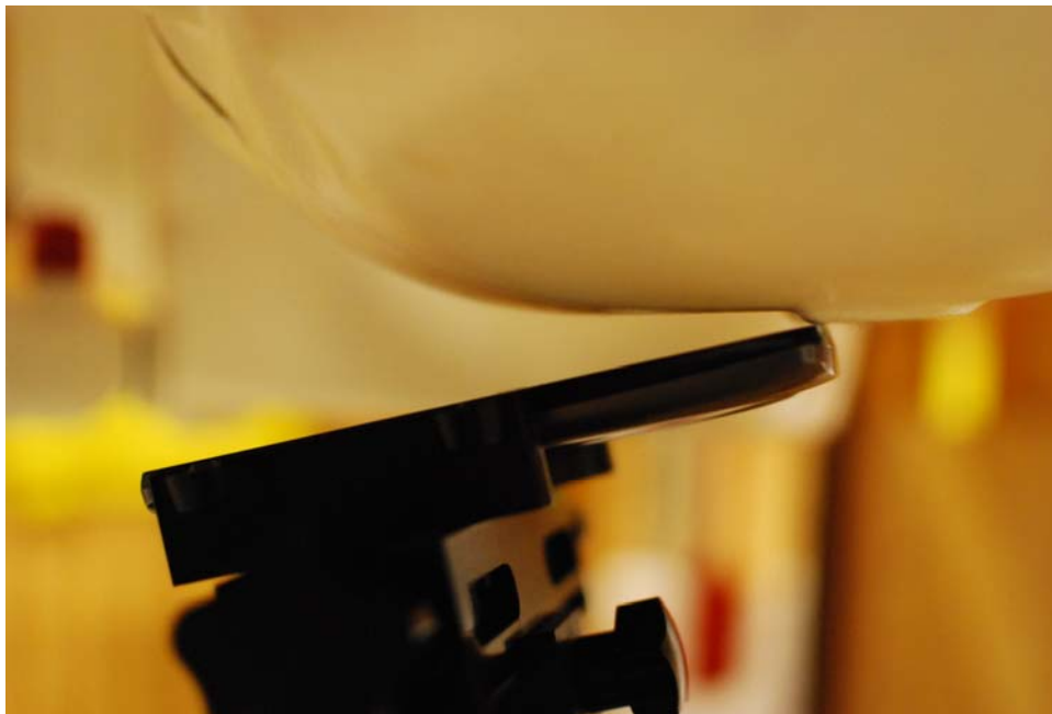
SAR Test Setup Photo 4 – Left Tilt
