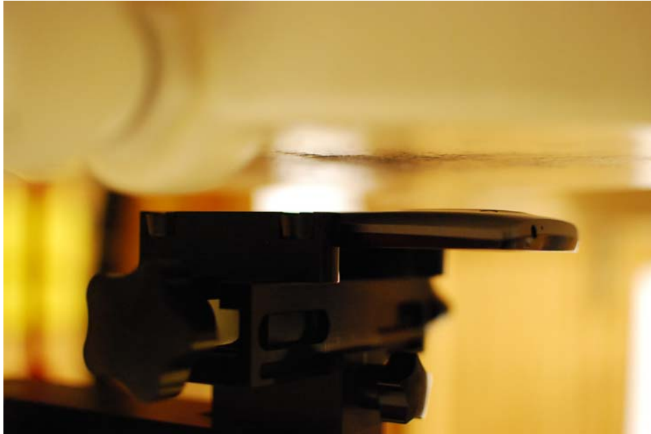
SAR Test Setup Photo 5: Body at 1.5 cm
