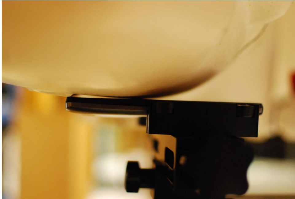
SAR Test Setup Photo 1: Right Cheek
