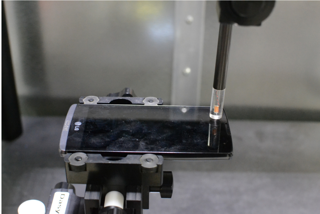
Figure 13-1 Test Setup for Wireless Device
