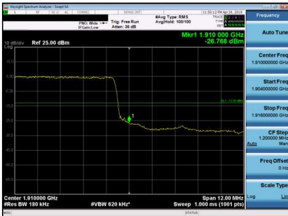
Plot 7-192. Upper Band Edge Plot (Band 2 - 15.0MHz QPSK - Full RB Configuration)
