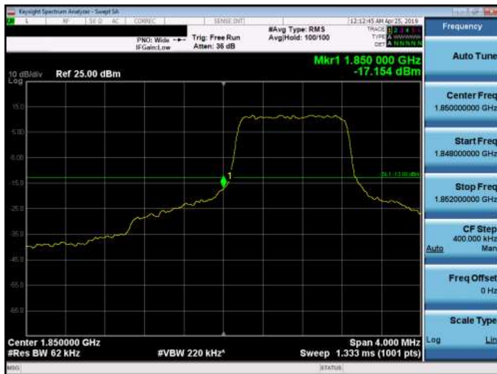
Plot 7-174. Lower Band Edge Plot (Band 2 - 1.4MHz QPSK - Full RB Configuration)
