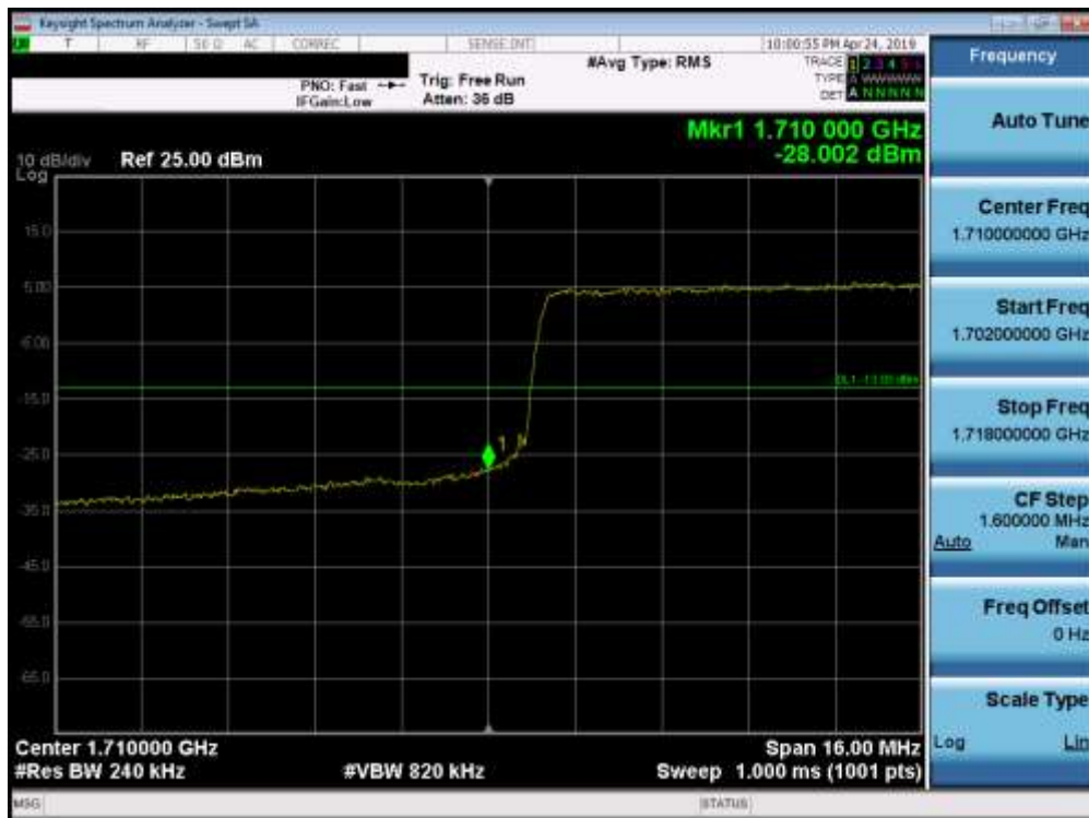
Plot 7-168. Lower Band Edge Plot (Band 66/4 - 20.0MHz QPSK - Full RB Configuration)
