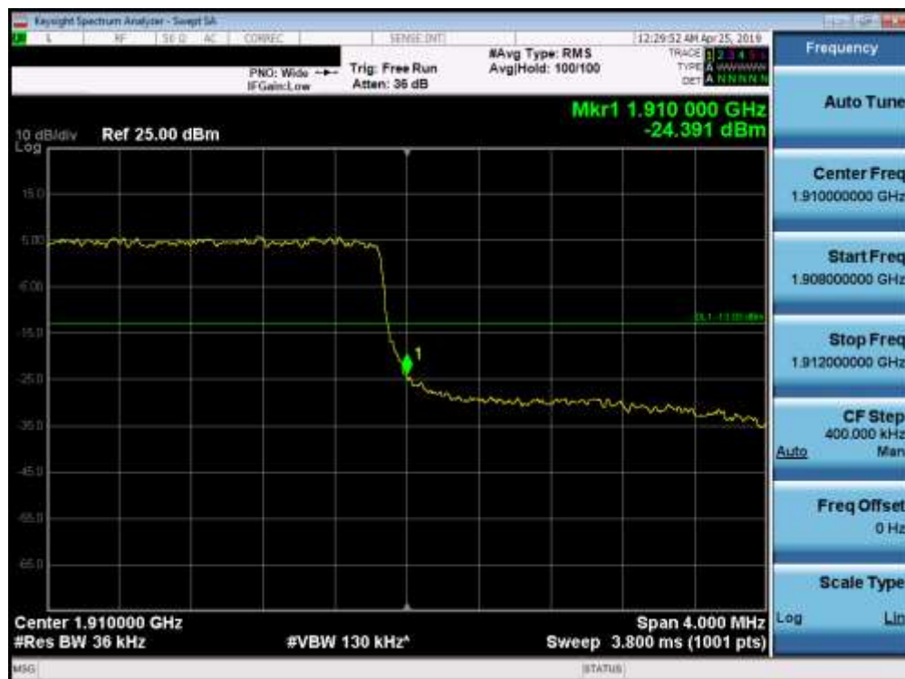
Plot 7-180. Upper Band Edge Plot (Band 2 - 3.0MHz QPSK - Full RB Configuration)
