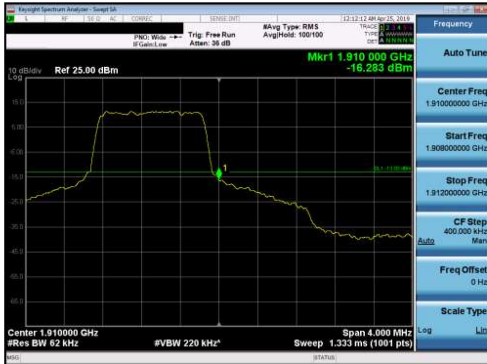
Plot 7-176. Upper Band Edge Plot (Band 2 - 1.4MHz QPSK - Full RB Configuration)
