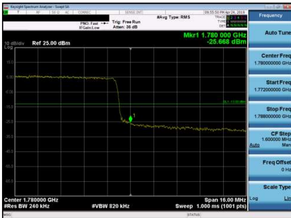
Plot 7-172. Upper Band Edge Plot (Band 66 - 20.0MHz QPSK - Full RB Configuration)
