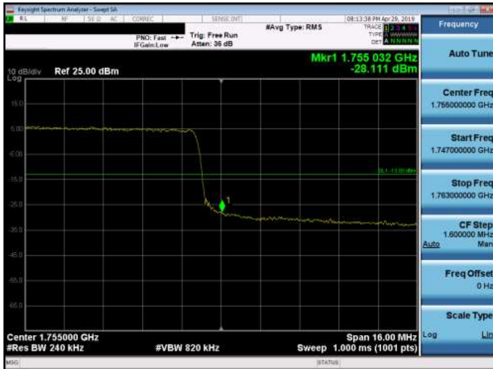
Plot 7-170. Upper Band Edge Plot (Band 4 - 20.0MHz QPSK - Full RB Configuration)
