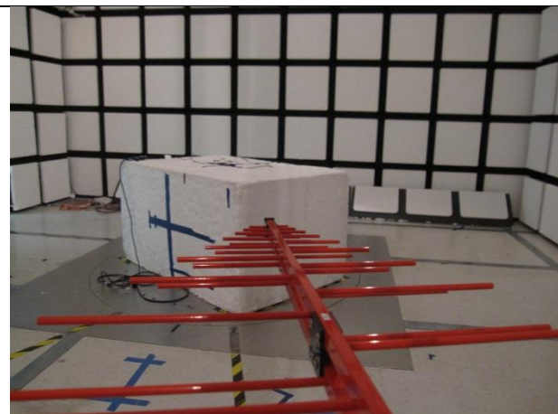
RADIATED FRONT PHOTO (BELOW 1 GHz)
