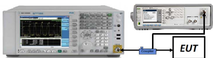
Figure 7-5. Test Instrument & Measurement Setup
