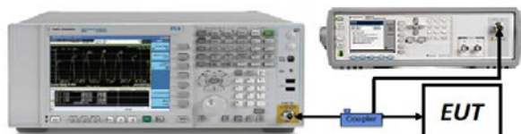
Figure 7-2. Test Instrument & Measurement Setup
