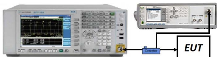
Figure 7-3. Test Instrument & Measurement Setup
