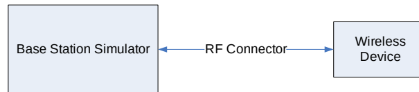
Figure 9-2 Power Measurement Setup
