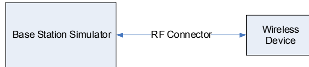
Figure 9-2 Power Measurement Setup
