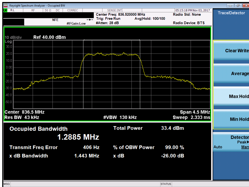
Plot 7-5. Occupied Bandwidth Plot (Cellular CDMA Mode)
