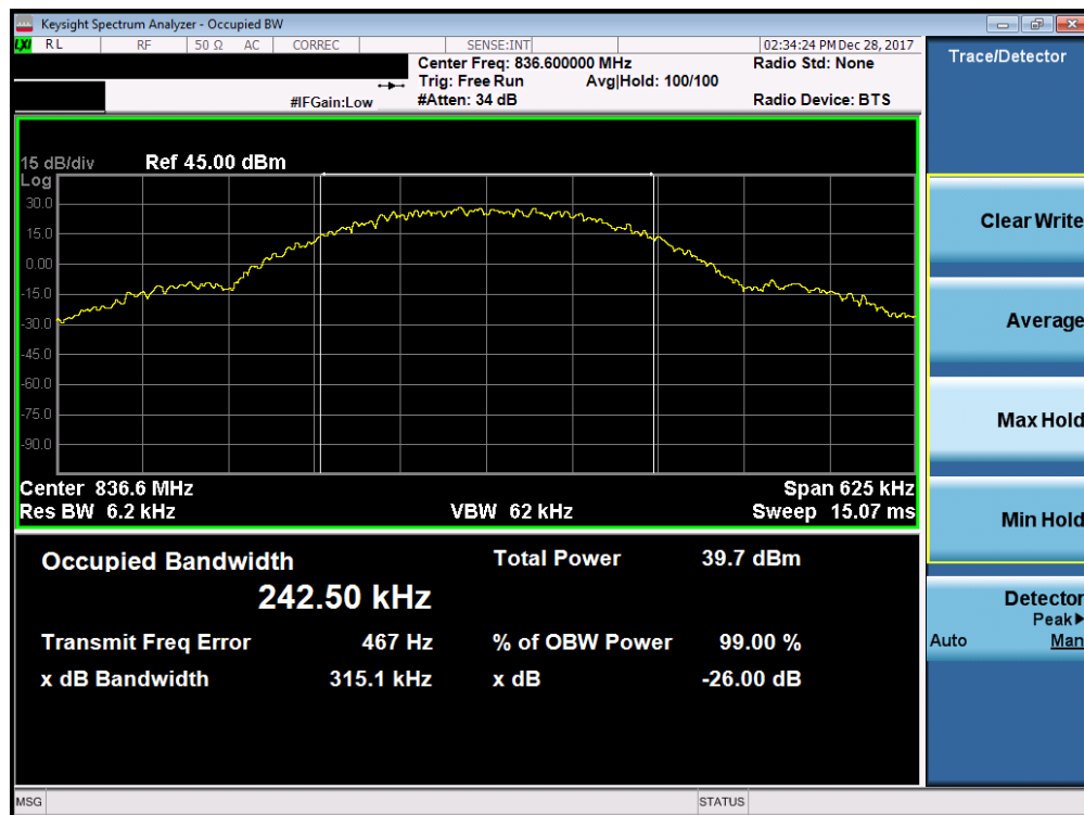
Plot 7-1. Occupied Bandwidth Plot (Cellular GPRS Mode)
