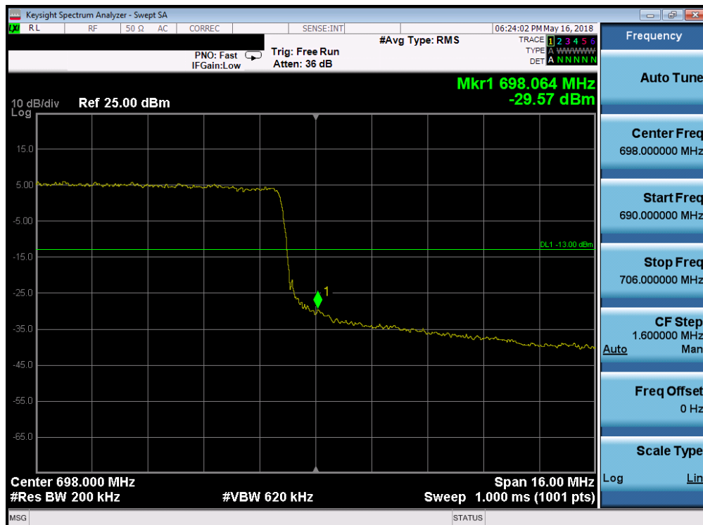
Plot 7-114. Upper Band Edge Plot (Band 71 - 20.0MHz QPSK - Full RB Configuration)
