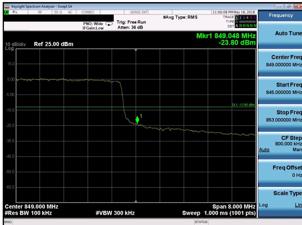
Plot 7-138. Upper Band Edge Plot (Band 5 - 10.0MHz QPSK - Full RB Configuration)
