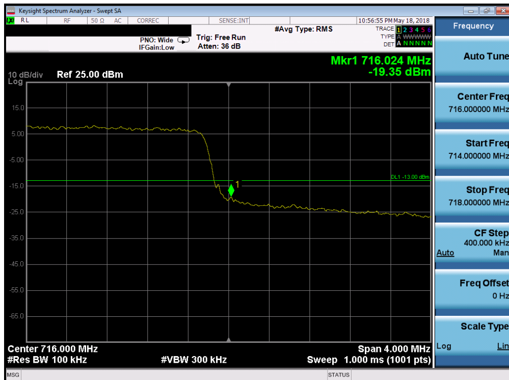
Plot 7-120. Upper Band Edge Plot (Band 12 - 5.0MHz QPSK - Full RB Configuration)
