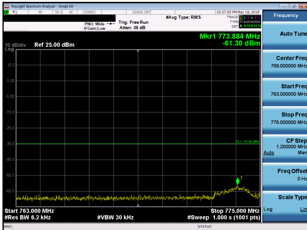
Plot 7-124. Lower Emission Mask (Band 13 - 5.0MHz QPSK - Full RB Configuration)
