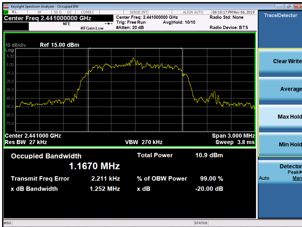
Plot 7-5. 20dB Bandwidth Plot (Bluetooth, 2Mbps – Ch. 39)
