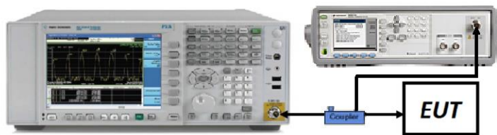
Figure 7-4. Test Instrument & Measurement Setup
